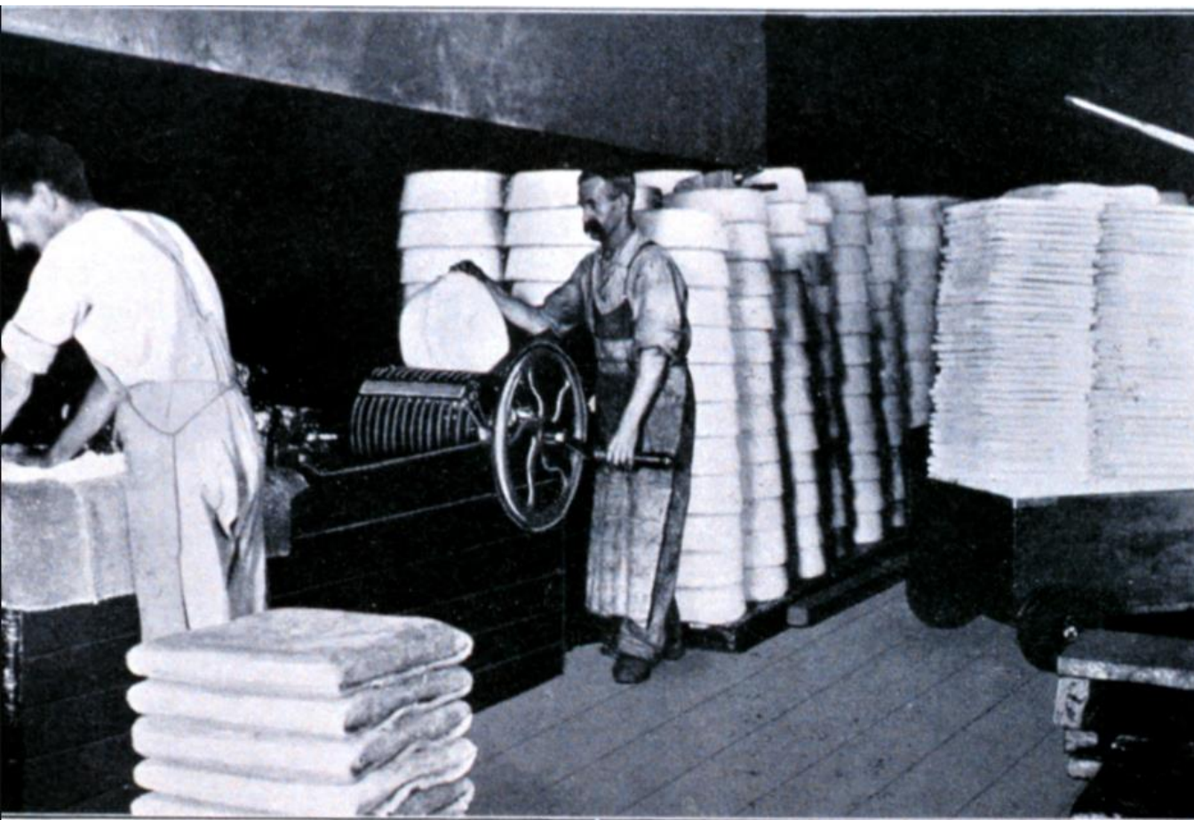
GRINDING AND PRESSING CRUDE SPERMACETI FOR REMOVAL OF TAUT-PRESSED OIL.
